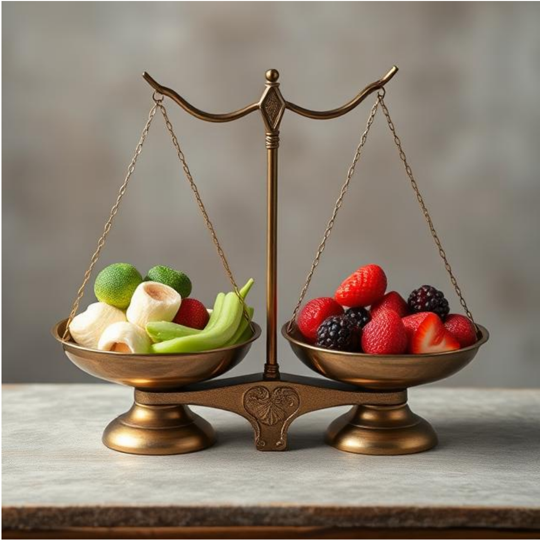
Figure 3: A two-pan balance in equilibrium, indicating that the mass on the left hand side equals that on the right hand side, even though the contents differ.
